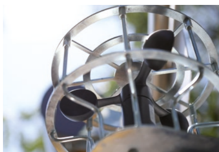
Anemometer for monitoring and warning that the maximum permissible wind speed (45km/h) has been reached
